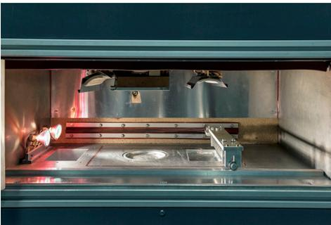
Mini-SLS-Bauraum [Foto: Fraunhofer UMSICHT]
