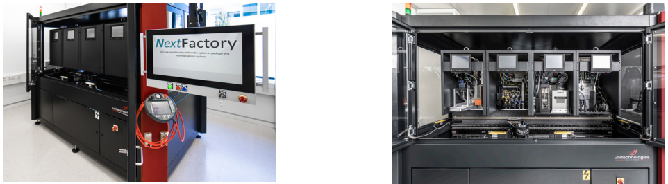
Fig. 1: NextFactory Machine (left) and its integrated modules (right): Inspection, assembly, curing and 3D-printing (from left to right) © Fraunhofer IPA
