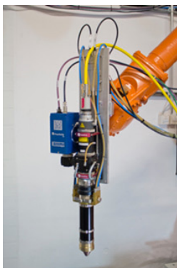
Fig. 1: Powder-based multi-material LMD processing (© Fraunhofer IWS)
