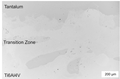
Fig. 3: Sharp material transition Ta/Ti6Al4V (© Fraunhofer IWS)
