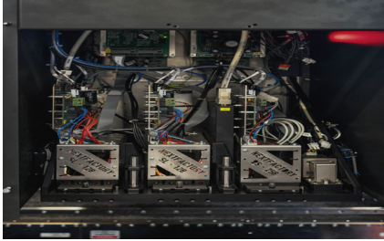
Fig. 2: Printing system containing 3 printing units, 2 UV-led light sources for pinning and a flattening unit (left); detailed bottom-view of printing unit (right) (© Fraunhofer IPA)
