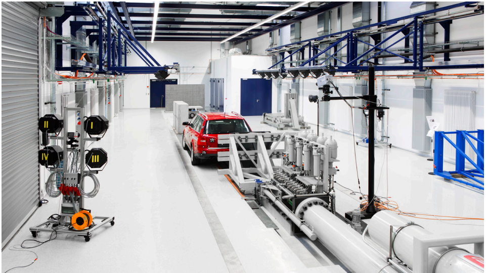
Full vehicle crash plant at EMI's laboratory location in Efringen-Kirchen (© Fraunhofer EMI)
