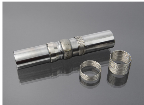
Figure 1: From right to left: positioning, cladding and finishing
