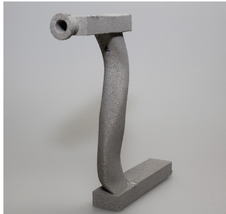
Complex shaped additive manufactured heat pipe sample © Fraunhofer EMI
