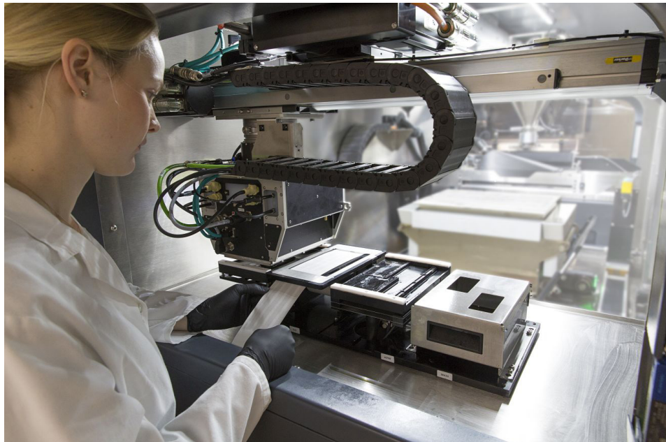
View into the new system for Metal Binder Jetting at Fraunhofer IFAM Bremen
