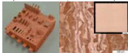
Figure 1: Pure copper benchmark geometry (left), microsection of 99,98 % dense sample (middle), microstructure of LPBF pure copper (right)
