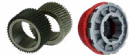
Figure 3: Prototype parts – PBF-printed and finished and coated test gear (left), extrusion printed gear body (right).
