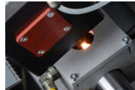
Figure 2: EW2C utilizes local shielding gas to ensure high cladding quality
