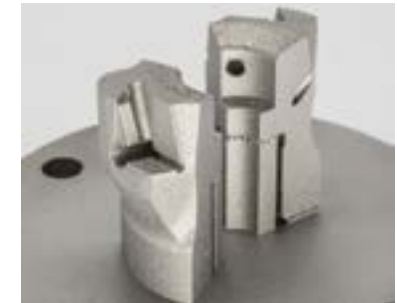
Cut-outs of an additively manufactured milling cutter head made of bainitic steel (Design: Sumitomo)
