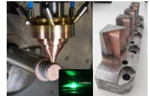
Figure 3: Laser Metal Deposition with green laser to build up multi material mould inserts (pure Cu / steel 1.2764)
