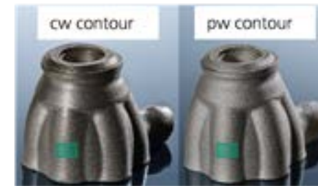
Figure 3: Macroscopic view of a turbomachinery part manufactured with cw (left) and pw (right) contour exposure
