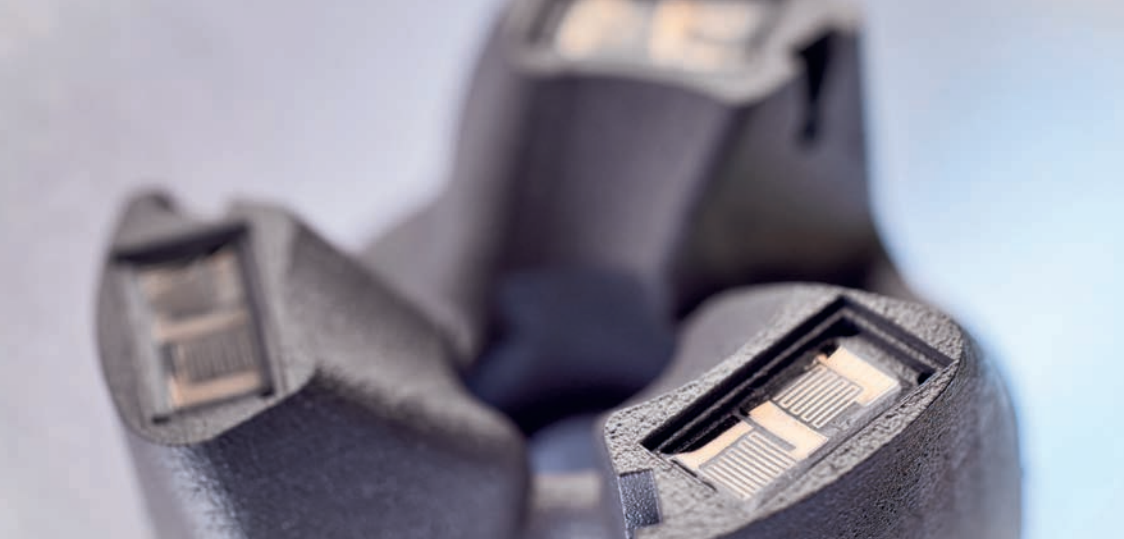
Strain gauges were integrated in a cutter head during the printing process. Left: The LPBF printing process is interrupted, and the printed strain gauges are fitted. Right: The printing process is continued to complete the intelligent component. © Fraunhofer IKTS
