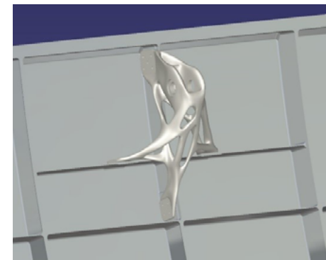
Figure 1: CAD model of the cargo aircraft door fitting with schematic illustration of the door structure
