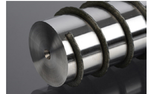
Figure 3: Welded spiral shape, Inconel 718 on 42CrMoV4, wall thickness 1.2 mm
