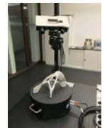
Figure 2: High-resolution 3D scan of the 3D printed cargo door fitting for quality assessment.
