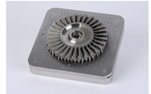
Figure 1: Clamping and referencing system for L-PBF and further processing
