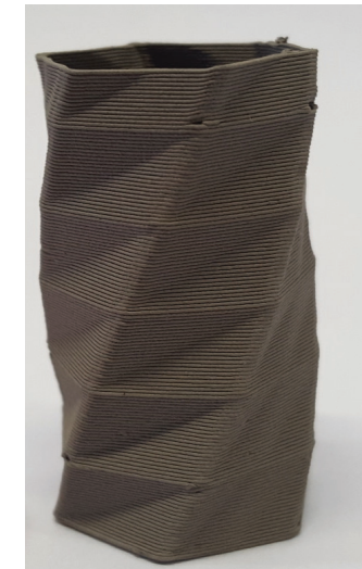
Fig. 3: greenbody SiC/SiC short fiber, \varnothing \sim 2 cm, h \sim 5 cm, CMC made by FFF (© Fraunhofer IKTS)
