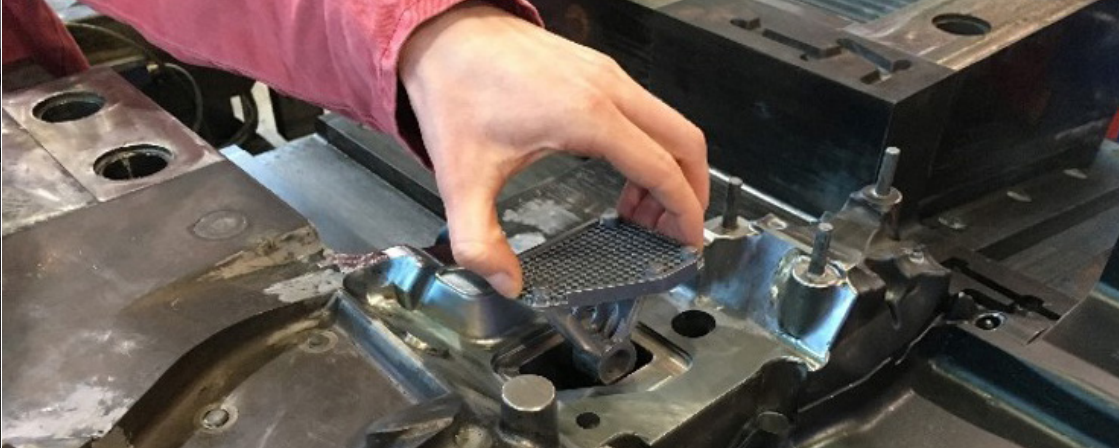
Optical measurement of 3D printed stainless steel reinforcement of die cast part (left), CastAutoGen demonstrators with EDAG concept car (centre), placement of aluminium adapter for power steering pump connector into the casting die (right)
