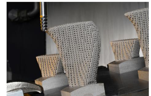
*Additive manufacturing enables low-vibration machining of components*
