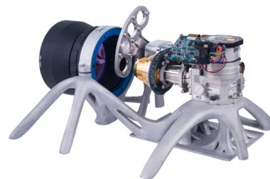
Fig. 1: 3D-printed optical bench of the nanosatellite ERNST
