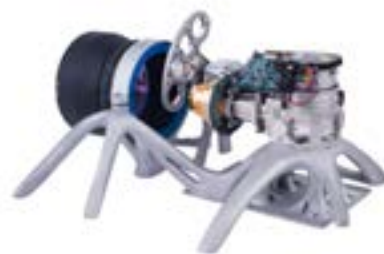
Fig. 1: 3D-printed optical bench of the nanosatellite ERNST
