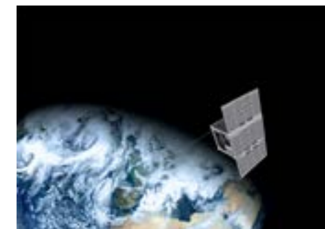
Fig. 3: In-orbit animation of the 12U nanosatellite ERNST
