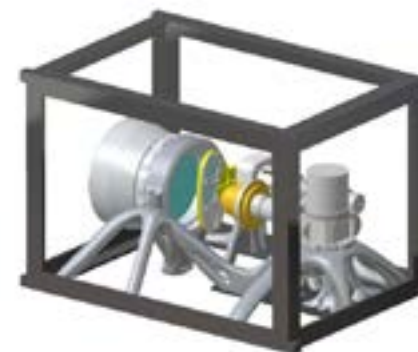
Fig. 2: Computer aided design of the integrated optical payload
