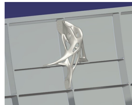
Figure 1: CAD model of the cargo aircraft door fitting with schematic illustration of the door structure
