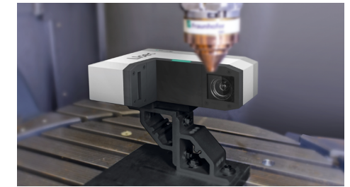
Figure 2: “Llsec” allows significantly simplified quality control and provides conclusions about the powder nozzle's wear degree.
