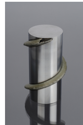
Figure 2: A cooling channel manufactured of Inconel 718, deposited onto 42CrMoV4 by the "LMD-W-20-L"
