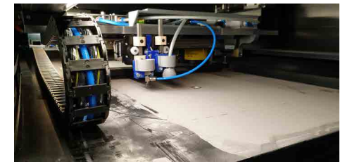
Kinematics for the integration of components during the laser beam melting process integrated in a laser beam melting plant
