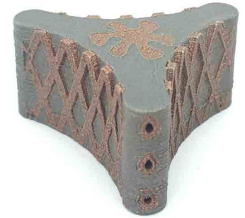
Multi-material component from the laser beam melting process made of tool steel and copper-chromium-zirconium
