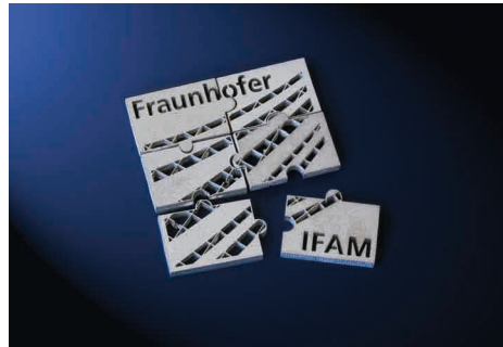
Demonstration part for additive manufacturing by 3D Metal Printing
