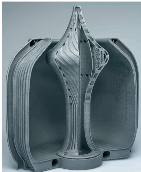
Rocket engine with aerospike manufactured by Laser Powder Bed Fusion
