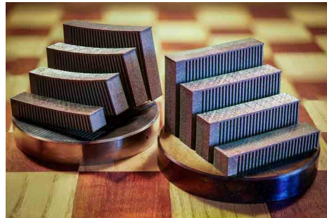
With an NIR emitter attached to the powder deposition unit, distortion in the component can be significantly reduced.
