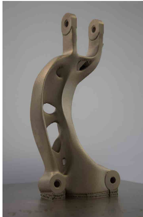
Resource-optimized design of a damper fork (automobile)
