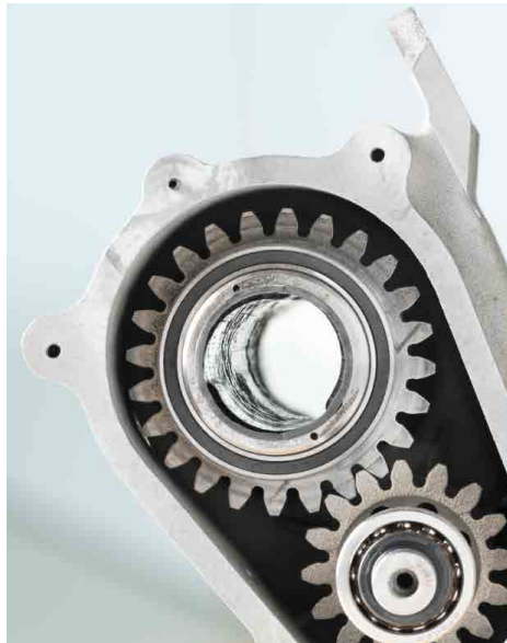
Multi-material gearbox; individual parts manufactured by additive manufacturing
