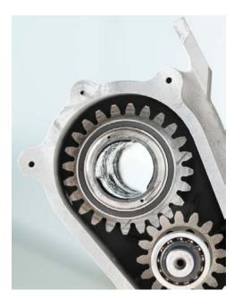
Multi-material gear; individual parts produced by additive manufacturing | ©Fraunhofer IGCV; Bernd Müller |
