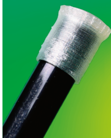
Shape transformation upon heating to 90 °C
